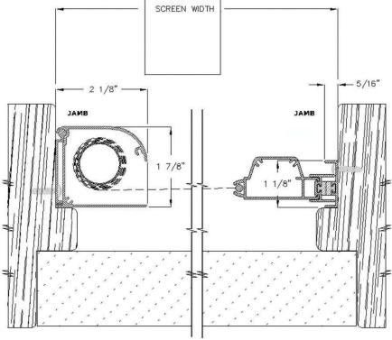
The dimensions for an Inside Mount Roll-Away® door are derived from the details at left (WIDTH) & (HEIGHT) above. Measuring by these dimensions will provide a door that will fit your opening.
