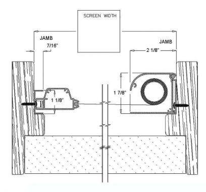
The dimensions for an Inside Mount Roll-Away® Door are derived from the details at left (WIDTH) & above (HEIGHT). Measuring by these dimensions will provide a door that will fit your opening.
